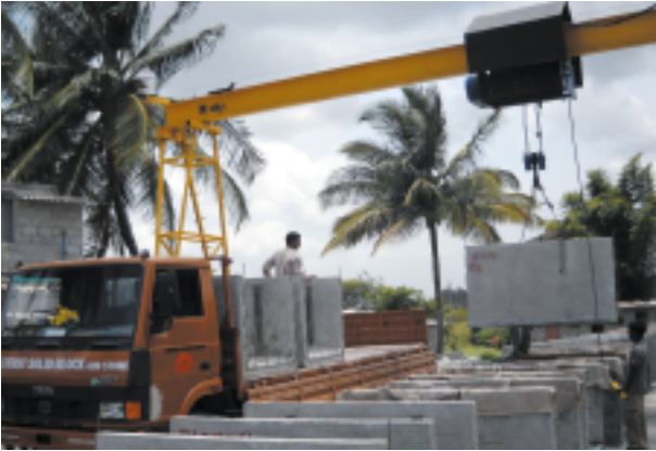
Loading of Trenches at factory by electrical Gantry
