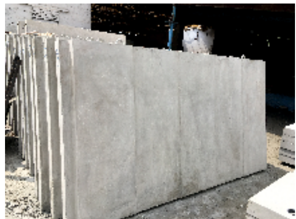
Stock of Wall Panel - I (2830x1500x80mm)
